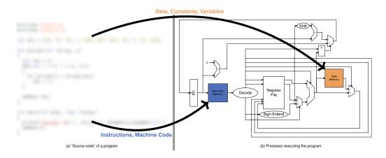
The compiler translates the source code, placing machine code (instructions) and data into memory.
