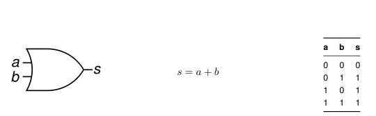
Note: x + 0 = x et x + 1 = 1, so an OR gate can be use to produce, from a signal x, a signal that equals to x or 1 depending on a command signal
